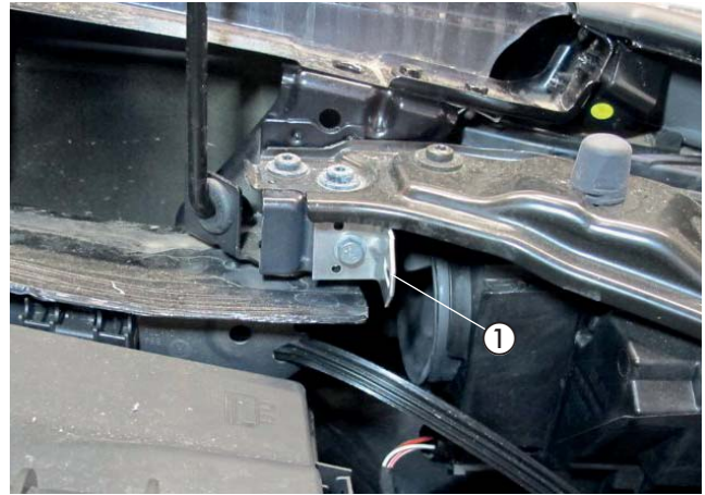
Fig. 43 ① 90° angle bracket mounted
