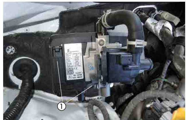
Fig. 23 ① Install heater
