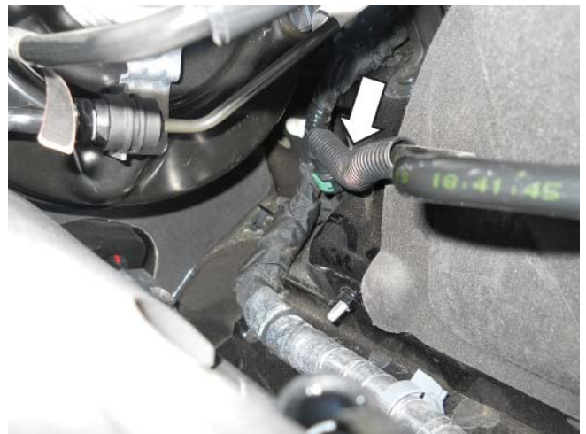
Disconnect green quick connect fitting
