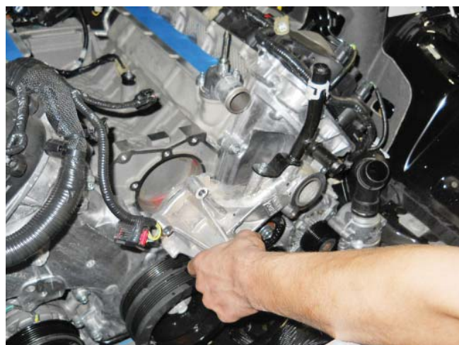
63. Place a clean towel in the water pump inlet cavity.
