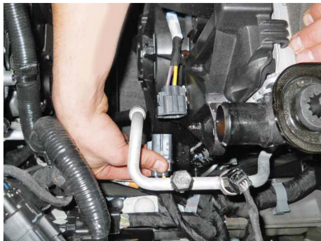
Fan shroud electrical connector
