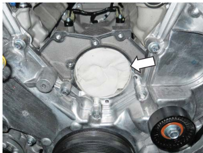
63. Place a clean towel in the water pump inlet cavity.
