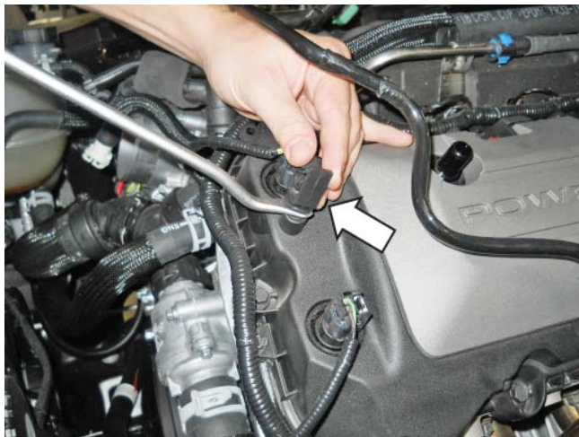
Remove retainer on cam cover
