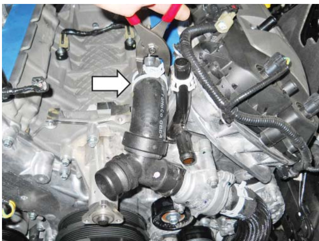
60. Remove the two (2) bolts from the thermostat housing (8 mm socket).
