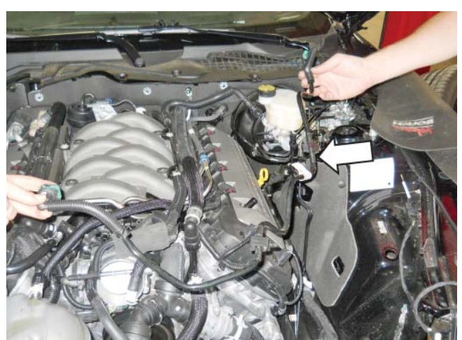
Disconnect green quick connect fitting
