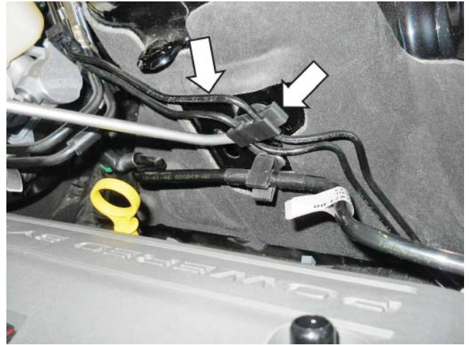
Remove tube from retainer
